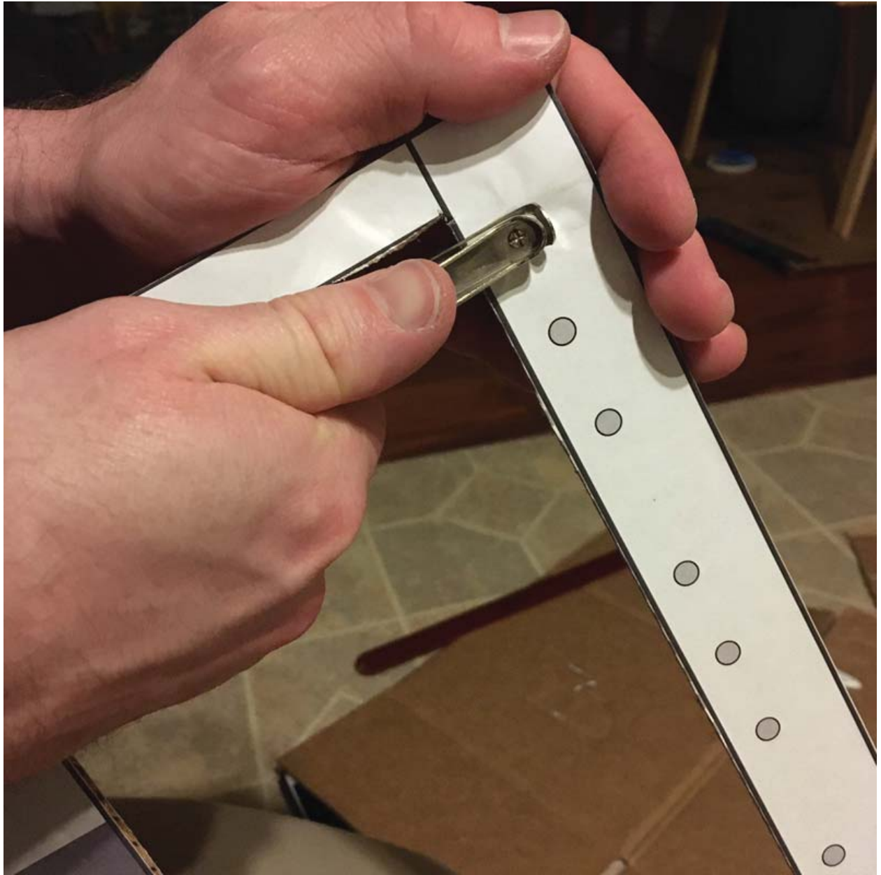
Step 6: Using a hole puncher, punch out each of the 14 holes (7 on each side).
